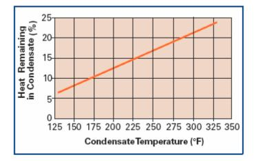
A simple calculation indicates that energy in the condensate can be more than 10% of the total steam energy content of a typical system.
