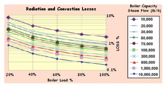
With modern boiler designs, this may represent only 1.5% on the gross calorific value at full rating, but will increase to around 6%, if the boiler operates at only 25 % output. Operating the boiler at full load will optimize this loss.
