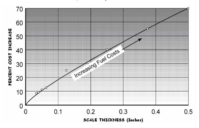
This brings out the importance of the scales and its influence on energy conservation in a boiler. It is intuitively obvious that the presence of any scale in a boiler is undesirable. The best way to deal with scale is not to let it form in the first place. Scale formation is prevented by:
